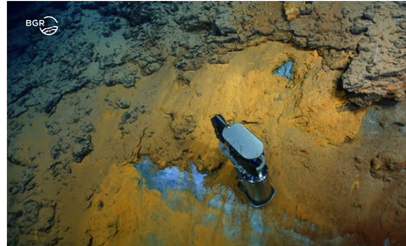
Surface of mound in JIM field with Fe-Mn crust disrupted exposing underlying massive sulphides. ATAP measurements
